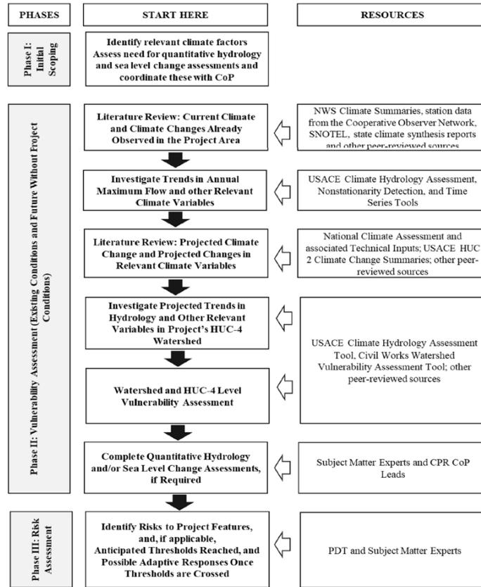
Figure 30. Flow chart describing steps for a qualitative assessment of impacts of climate change in hydrologic analysis (ECB 2018-14)
