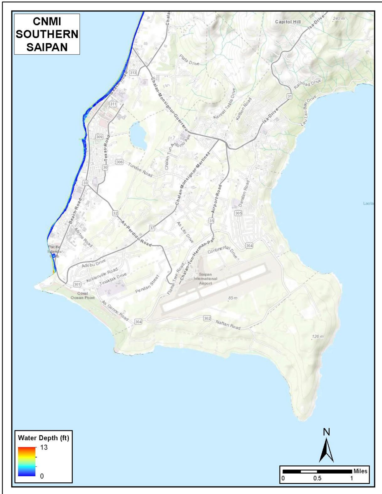
Figure 48. Southern Saipan, 1% AEP Coastal Flooding, Future Conditions
